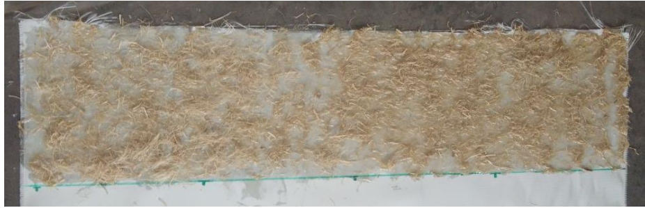
FIG.16 Spreading of the Epoxy Paste over the E-glass fabric
