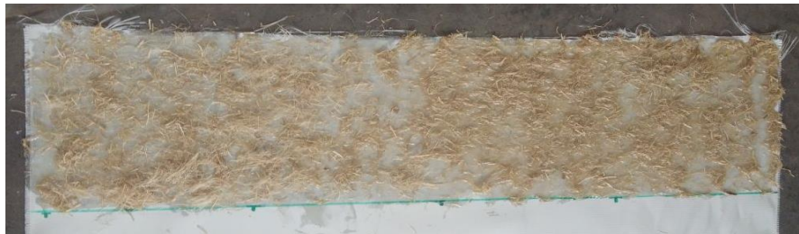
FIG.23 Spreading of The Epoxy Paste Over The E-Glass
