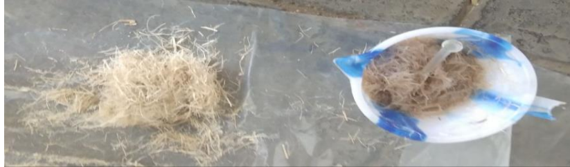
FIG.13 Mixing of Short Banana Fiber with Epoxy Resin Mixture
