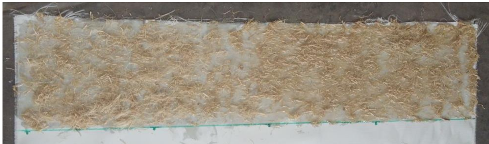
FIG.27 Spreading of the Epoxy Paste over the E-glass fabric
