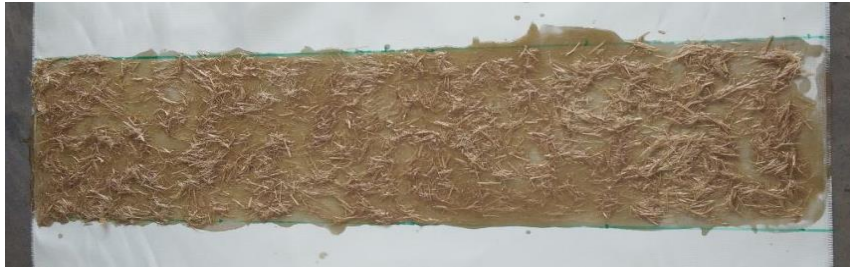
FIG.17 Spreading of The Phenolic Paste Over The E-Glass Fabric
