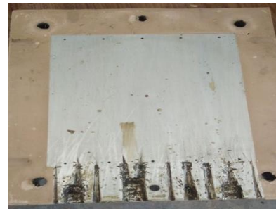
FIG.14 Mold Cavity Filled with Mixture of Epoxy and Banana Fiber
