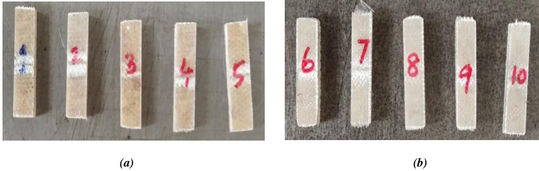
FIG.31 Tested Specimens of ILSS (a) E-glass/Banana fiber with Epoxy/Phenolic Resin Tested Specimens (b) E-glass/Banana fiber with Epoxy Resin Tested Specimens
