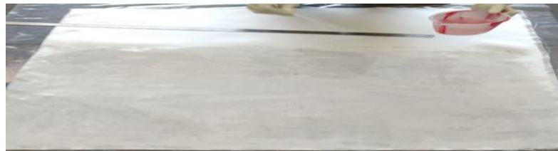
FIG.6 E-glass Fabric with Epoxy Resin Hand Layup
