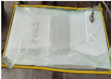
FIG.8 Vacuum Bagging of Laminates
