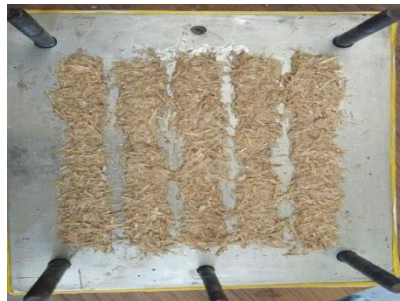
FIG.14 Mold Cavity Filled with Mixture of Epoxy and Banana Fiber
